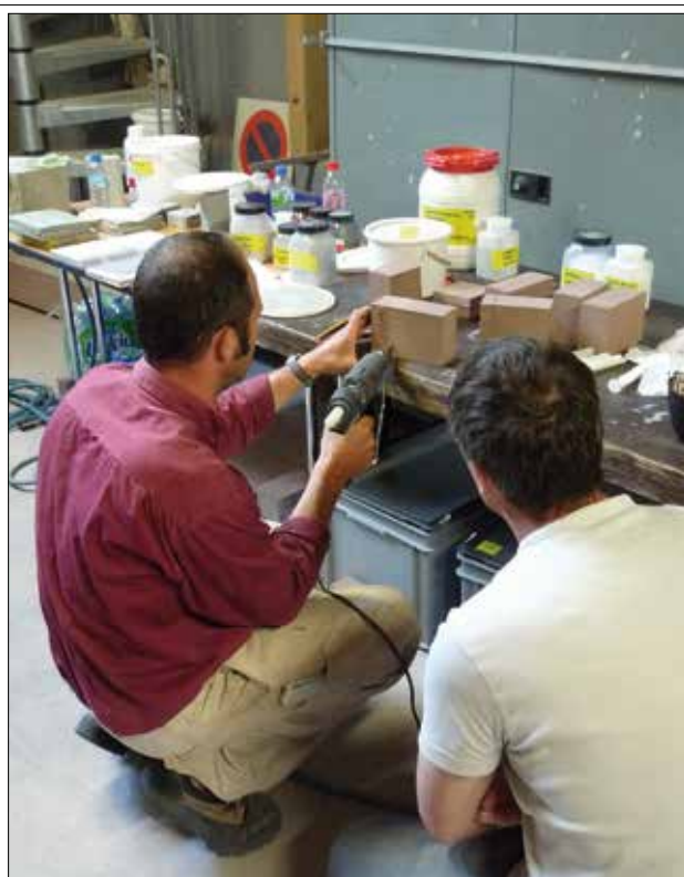
Figure 4 : Percer sans percussion
